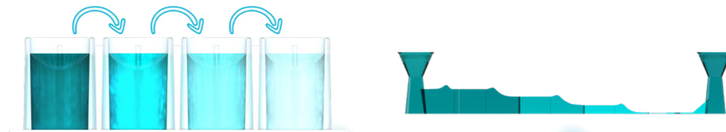
Comparison of dilutions in standard wells and physical dilution in SpecPlate measurement chambers by path length variation (SpecPlate structure rolled out for demonstration purposes)
