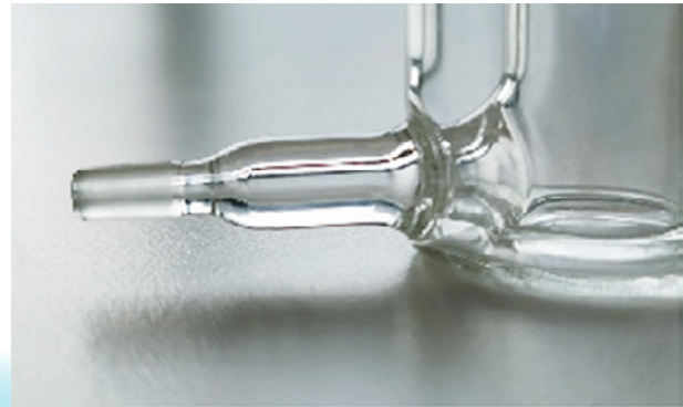
Partial/full sampling Updated Franz cell design can perform partial or full sampling
