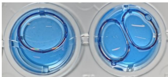
Figure 1 Air bubbles in the well of a standard plate after pipetting Bradford Solution
